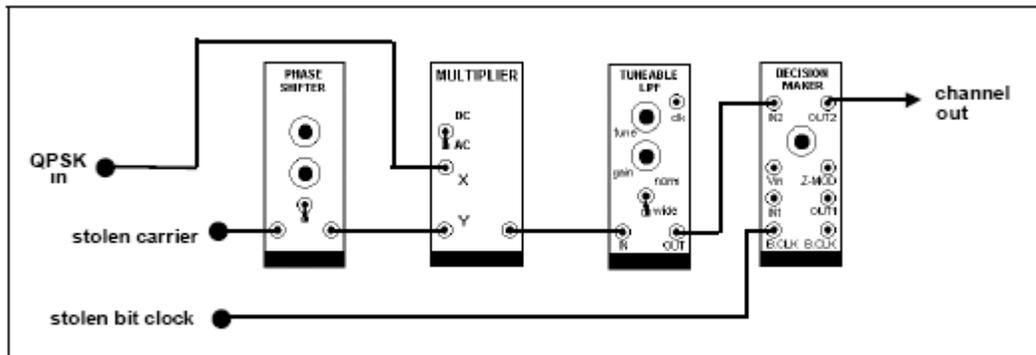
**Figure 5: one channel of the demodulator**
