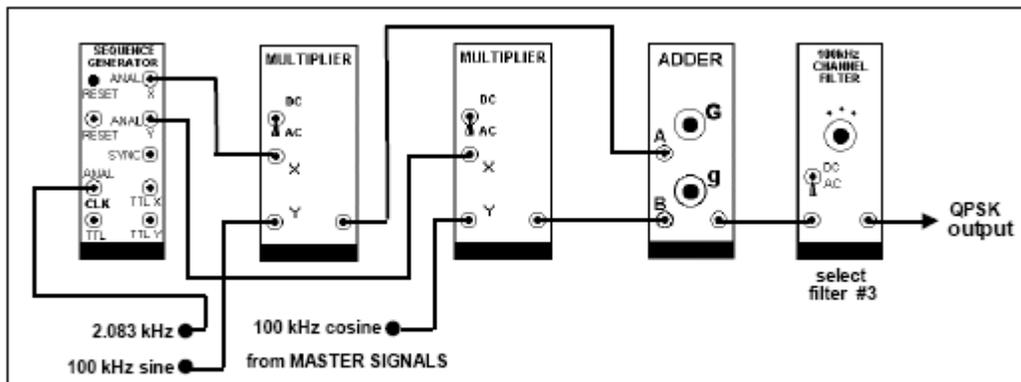
**Figure 4: the QAM modulator for QPSK**
