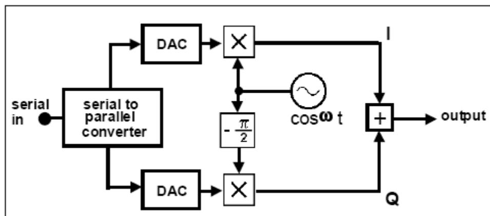
**Figure 2: a QPSK modulator**
