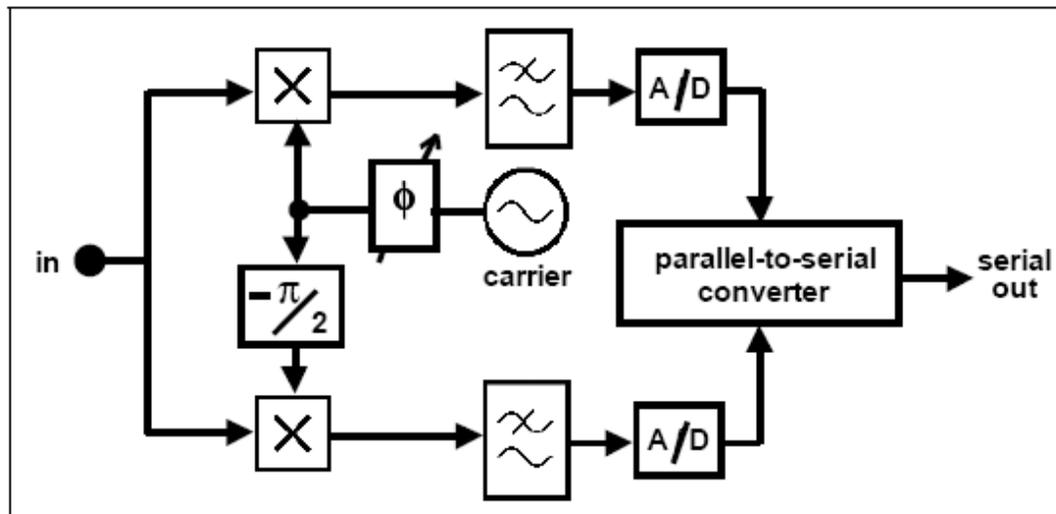
**Figure 3: the QAM demodulator for QPSK**
