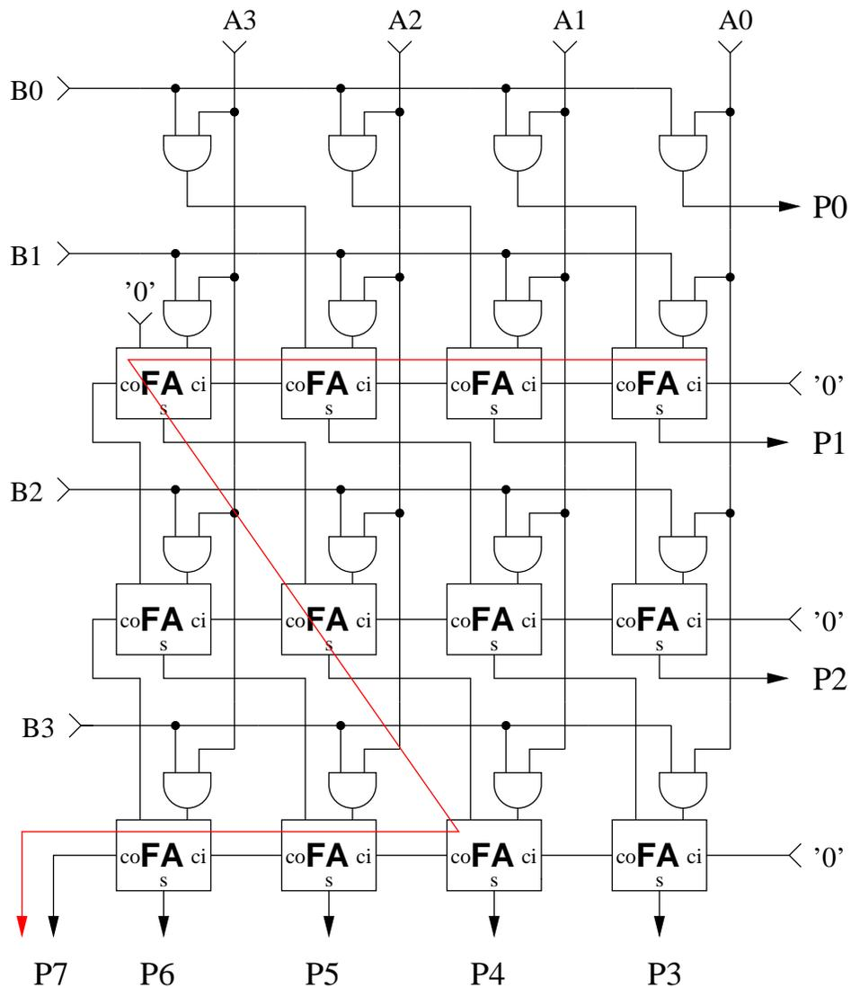
Worst Case Propagation Delay:  $T_{pd} = [3N-4] \cdot t_{pd}(FA)$
