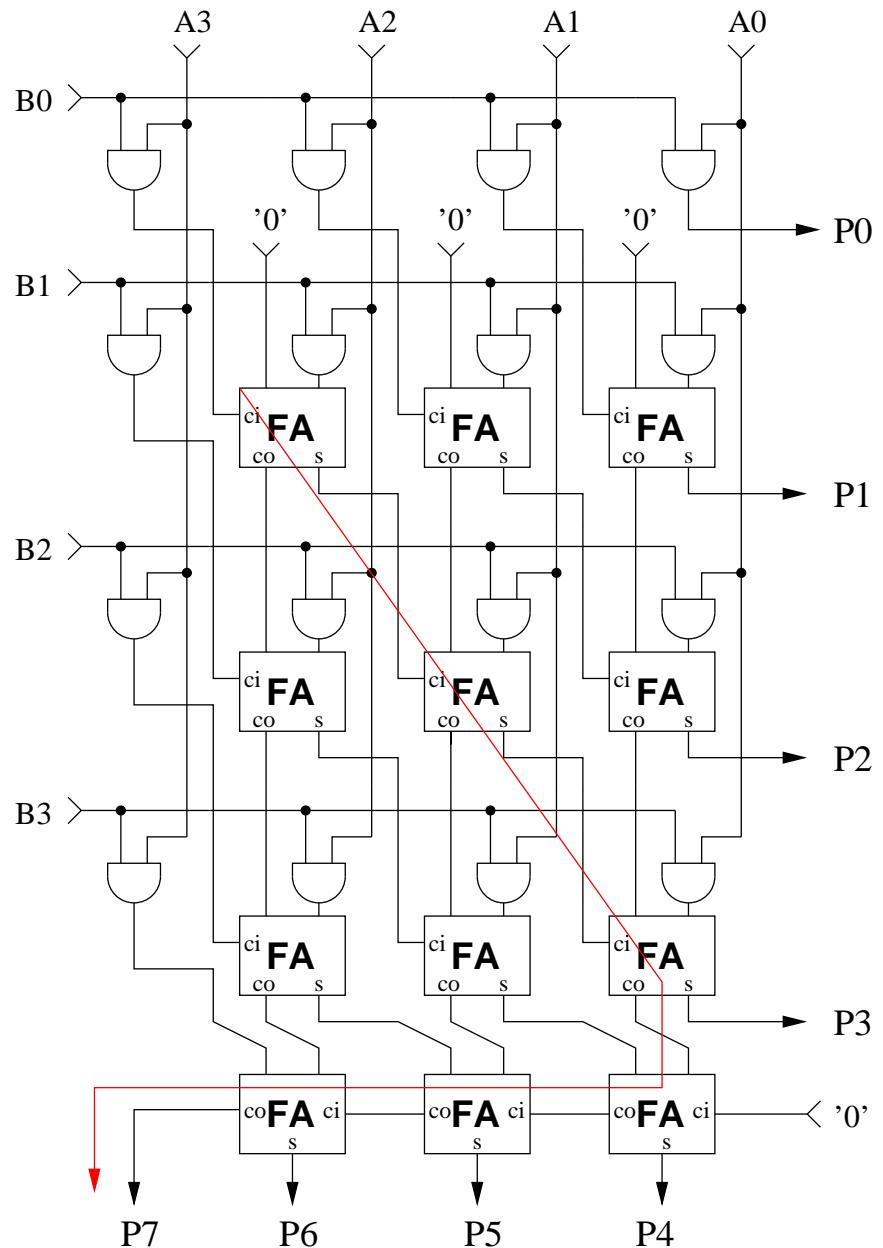
Worst Case Propagation Delay:  $T_{pd} = [2N-2] * t_{pd}(FA)$
