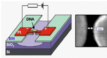
In this experiment, 10.4 nm long DNA molecules, each DNA molecule with 30 base pairs, are connected to two metal nano electrodes by electrostatic trapping. Current is absorbed across the electrodes.
