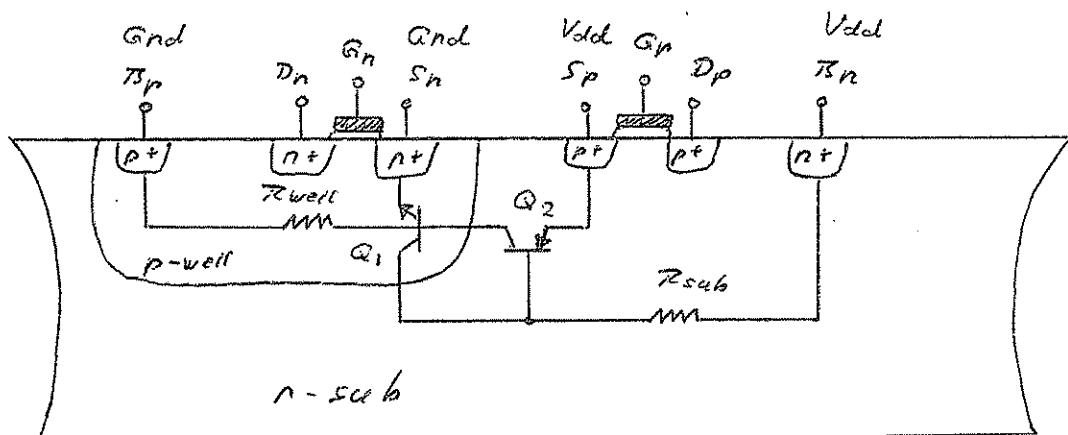
$Q_1$ : vertical npp transistor ( $n$ -sub / p-well /  $s_n$ )
