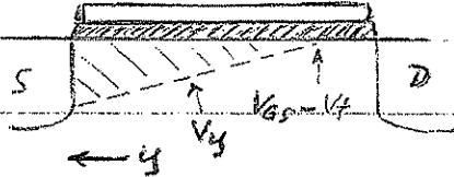
b)  $C_{ADS} = \frac{\partial Q_f}{\partial V_{GD}} \approx 0$  (except for very small  $L$ )
