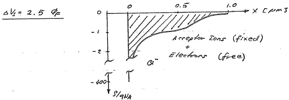
Note: The free charge carriers created through accumulation (holes in p-Si) or inversion (el in p-Si) reside in an extremely narrow portion of the semiconductor immediately adjacent to the oxide layer. By comparison, the depletion region (acceptor ions in p-Si) extends much deeper into the semiconductor.
