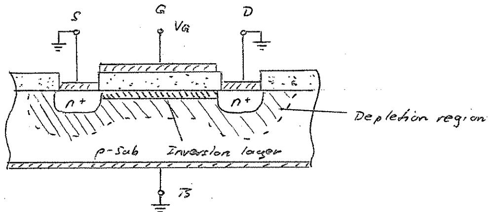
Threshold voltage  $V_T$ : ( $V_{SB} = 0$ )
