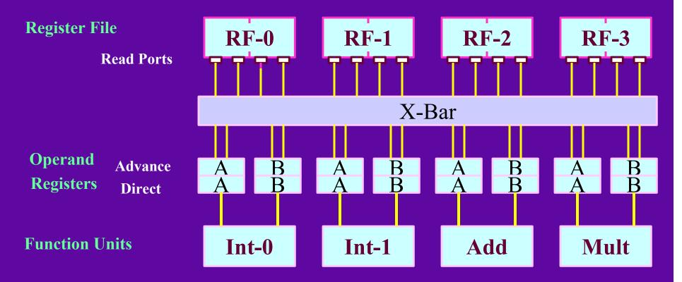
Port 0 supplies Operand A; Port 1 supplies Operand B.Port 3 is used to read registers for store transfers.
