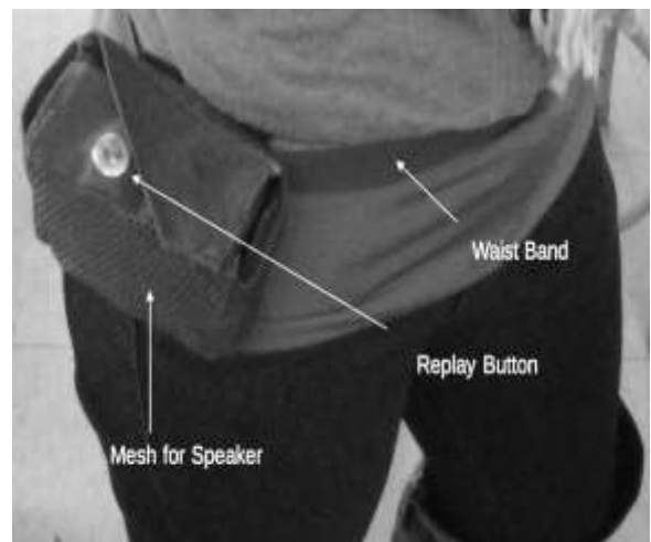
60 Fig. 1. The mobile unit of the Activity Analyzer in a carrying pouch strapped around the waist.
