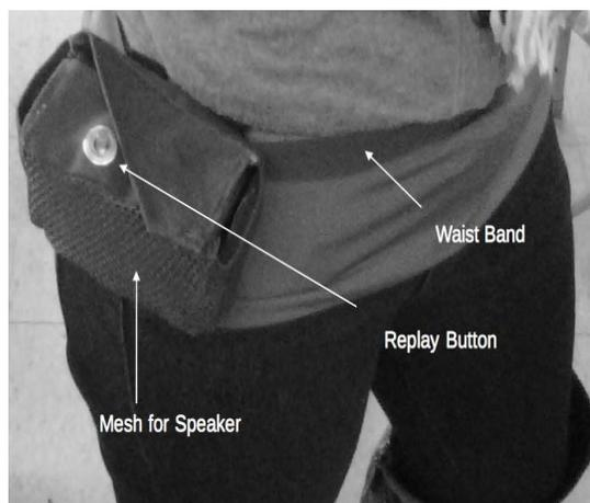
Fig. 1. The mobile unit of the Activity Analyzer in a carrying pouch strapped around the waist.
