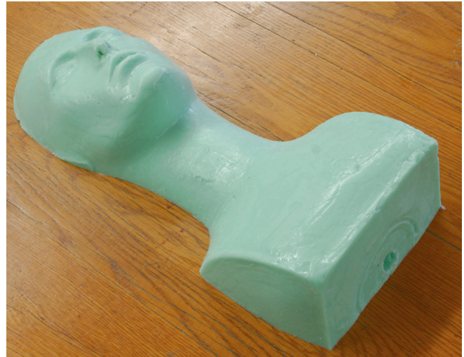
Figure 3. The silicone-rubber head model that has a void inside representing the tracheal, mouth and nasal chambers.
