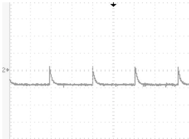
Figure 3. Action potentials generated from the neuron emulator, seen at the D/A. Testing of the device was performed to ensure functionality.
