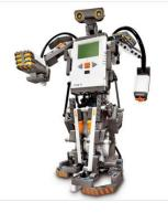
Our goal is to combine SEMG with a PIC microprocessor using a wireless Bluetooth connection, using the previously established algorithms to detect the peaks of the muscle contractions and their strength, which in turn is sent to the LEGO Mindstorm NXT which controls the movements of the LEGO
