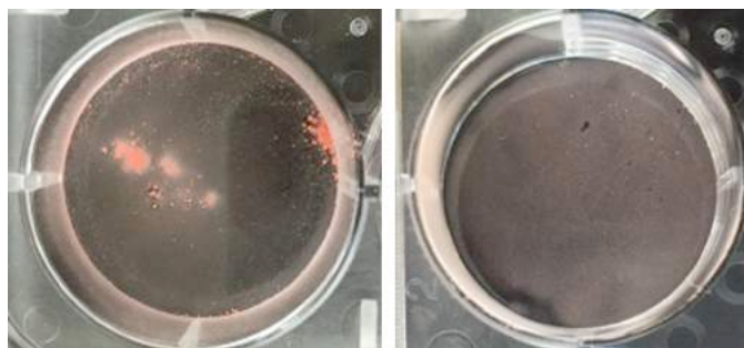
Fig. 2. A model red powder injected into a Transwell® resulted in a clustering pattern without using the dispersion device (left) and a uniform pattern with the dispersion device (right).
