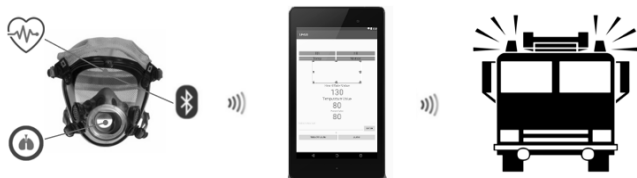
Fig. 1. bPASS Data Flow – physiological data is relayed to the Android phone. Any triggered alarms would be heard audibly and relayed to a local base station.
