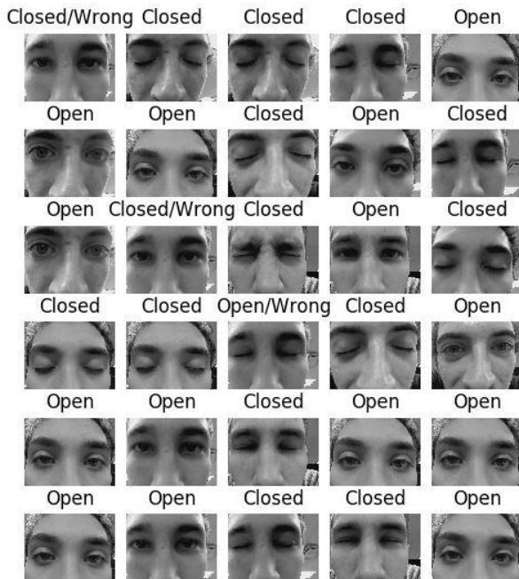
Fig. 2. 30 grayscale images tested against the machine learning algorithm. The eye status of 27 of the 30 images was successfully determined.
