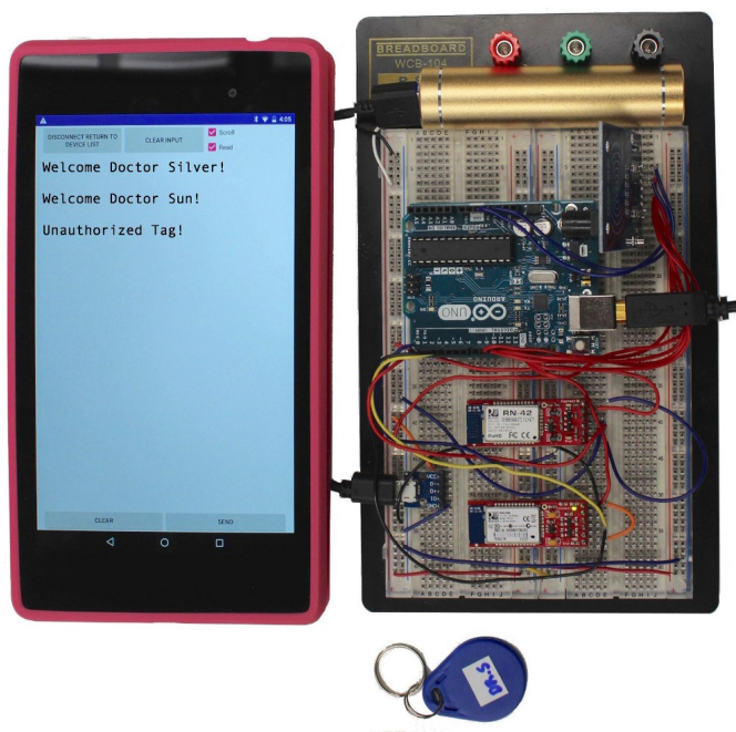
Figure 2: The functional prototype of the RFID-smartphone based personnel tracking system. During the development, an Android tablet was used instead of a smartphone.
