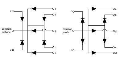
and to allow for multiplex operation (more on this at a later date). For use in a circuit, the device's normal pin connections are shown below for both types of device. The first thing that you should do is identify which one you have in your kit.
