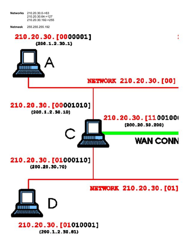
We have expanded the last byte of the IP address so that we can show the network subaddressing. The standard IP address nomeclature is shown below this expanded version.
