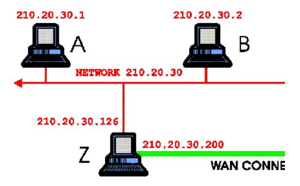
Node A is one of the many workstations on the Ethernet segment Net 0. Node Z is a JBM unit and the gateway from this Ethernet to the Internet service provider's gateway machine G. Some of the other workstations have been labeled as B to Y for illustration, but will not be referred to in this example as their setup will be the same as for A.
