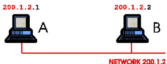
In the diagram above and subsequent diagrams, we have emphasized the network number portion of the IP address.
