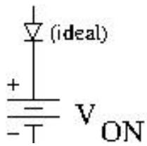
Constant Voltage Source Equivalent Circuit. ( $V_{ON}=0.7V$ )
