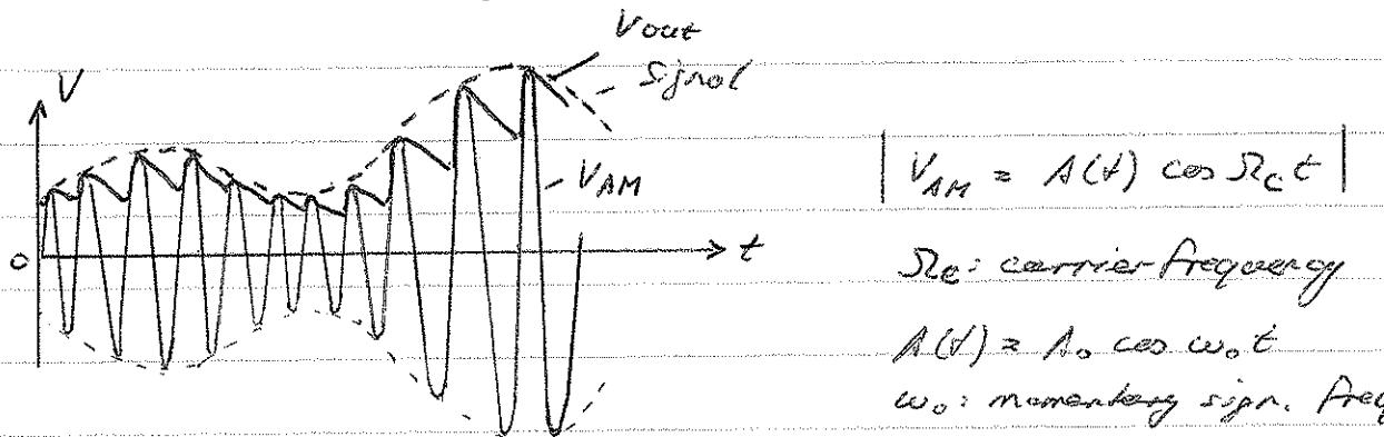
The  $RC$  time constant  $\tau$  of the detector must be chosen such that the maximum slope of the output voltage is at least as large as the maximum slope of the envelope, i.e. the AM input signal before modulation.
