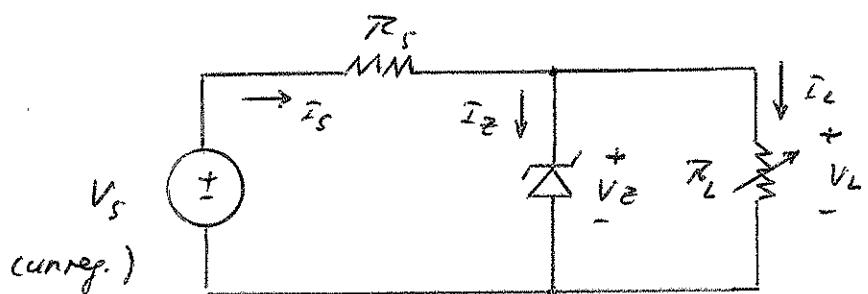
A voltage regulator can be used to remove a ripple from an input voltage and (or) to maintain a const. output voltage over a range of loads.
