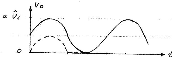
Cascade of clamping circuit with simple rectifier
