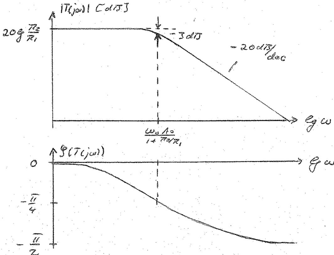
Example 4a Noninverting amplifier with
