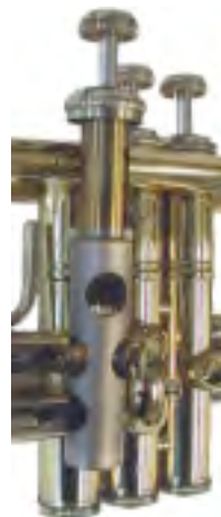
Figure 6.12: Each trumpet valve has two paths through which air can flow. When the valve is not depressed, it allows air to flow through the primary tube. When the valve is depressed, air is forced through different chambers that divert it through an additional length of tube. This additional length causes the standing sound wave to be longer and its frequency to be lower.
