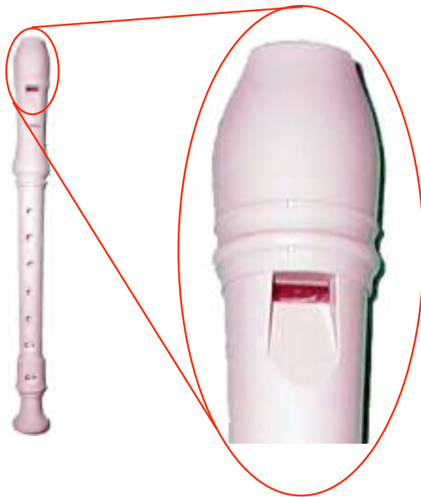
Figure 6.5: The “air reed.” A portion of the air stream entering the recorder moves down the tube and reflects back from its open end, as in the case of other wind instruments. However, rather than interrupting the air stream mechanically with a mechanical reed or with the lips of the player, the reflected air pulse itself acts as a reed. The low and high-pressure portions of this sound wave in the recorder interrupt the player’s air stream, causing it to oscillate in and out of the instrument at the same frequency as the standing sound wave.
