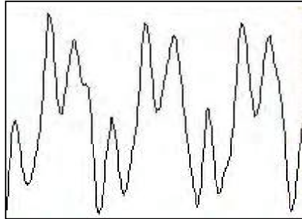
Figure 3.4: The complicated waveform shown here is typical of that produced by a musical instrument. This waveform can be produced by combining the waveform of the fundamental frequency with waveforms having frequencies that are integer multiples of the fundamental frequency.
