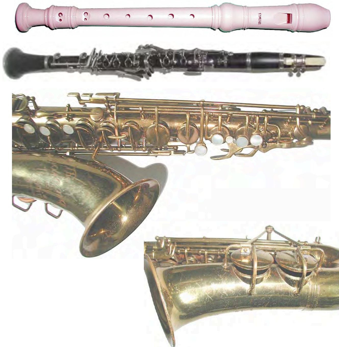
Figure 6.15: From the recorder to the clarinet to the saxophone, tone holes go from small and simple to small and complex to large and complex. As the instrument grows in length and diameter, the tone holes get further apart and must also grow in diameter. Compare the simple tone holes of the recorder, which can be easily covered with the player's fingers to the tone holes of the saxophone, which must be covered with sophisticated multiple, large diameter hole closer systems.
