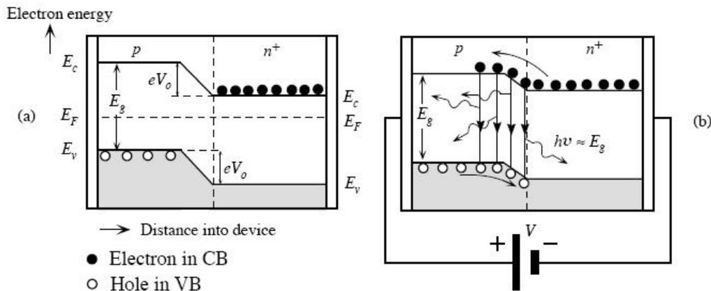
(a) The energy band diagram of a  $pn^+$  (heavily  $n$ -type doped) junction without any bias. Built-in potential  $V_0$  prevents electrons from diffusing from  $n^+$  to  $p$  side. (b) The applied bias reduces  $V_0$  and thereby allows electrons to diffuse or be injected into the  $p$ -side. Recombination around the junction and within the diffusion length of the electrons in the  $p$ -side leads to photon emission.
