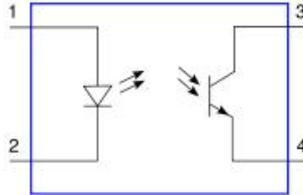
**Figure 5: Optocoupler schematic showing LED and phototransistor (Wikipedia)**
