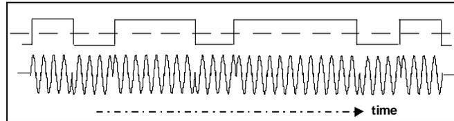
**Figure 2: a BPSK signal in the time domain.**
