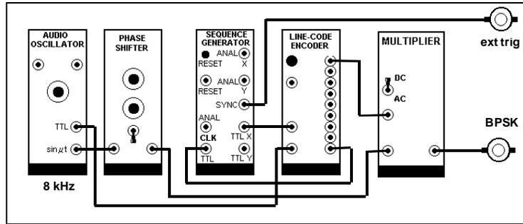
**Figure 5: model of the BPSK generator**
