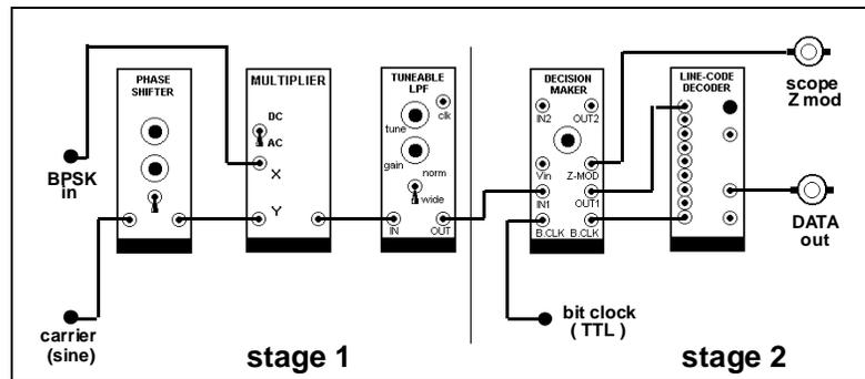
**Figure 6: the BPSK demodulator**
