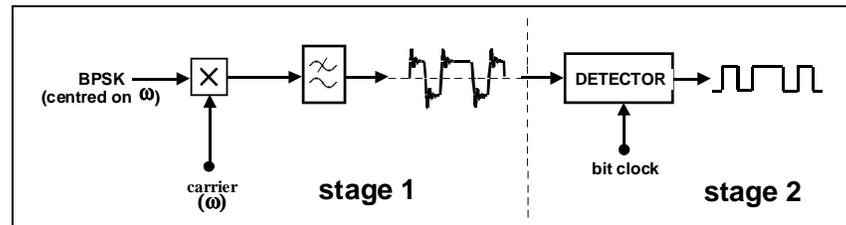
**Figure 3: synchronous demodulation of BPSK**
