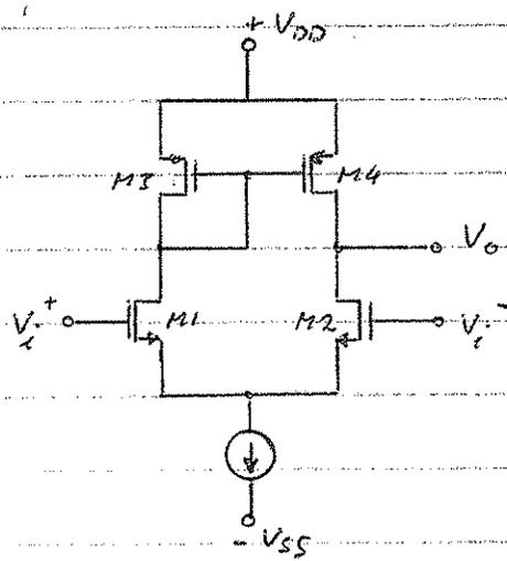
1. replace circuit elements by noiseless elements and their equivalent noise sources.
