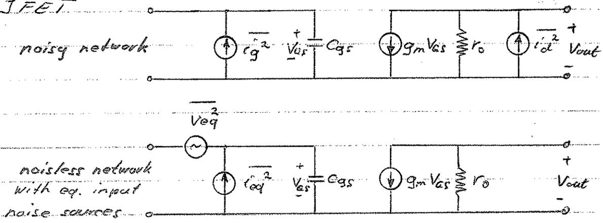
A) Short inputs to find  $\overline{v_{eq}^2}$
