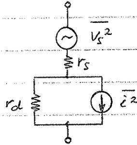
1.  $r_d = \left[ \frac{dI_D}{dV_D} \right]^{-1} = \frac{kT}{qI_D}$  Modelling resistor (produces no noise)
