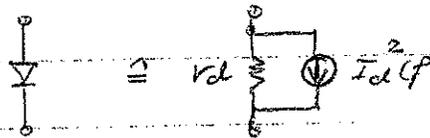
$$r_d \approx \frac{\eta V}{q I_D} \quad I_d^2(f) \approx 2q I_D$$
