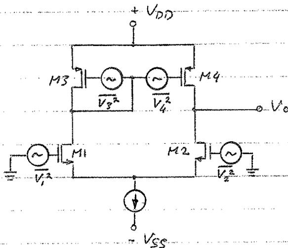
Output noise power: (assume  $\overline{V_1^2} = \overline{V_2^2}$  and  $\overline{V_3^2} = \overline{V_4^2}$ )
