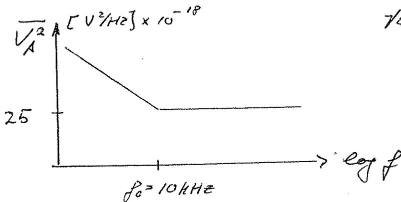
Question: What is the total noise power in the frequency band from 10 Hz to 100 kHz?
