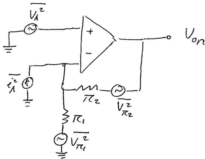
$$\| V_{on}^2 = \overline{V_A^2} \left(1 + \frac{R_2}{R_1}\right)^2 + \overline{e_A^2} R_2^2 + \overline{V_{R_1}^2} \frac{R_2^2}{R_1^2} + \overline{V_{R_2}^2} \|$$
