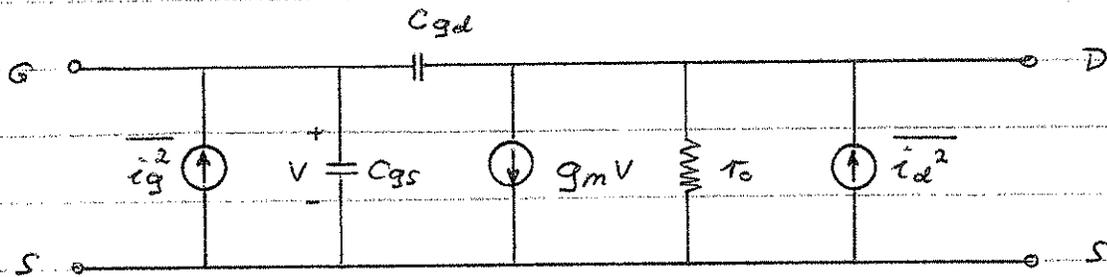
1.  $\overline{i_g^2} = 2qI_G \Delta f$  Shot Noise due to reverse leakage in JFET
