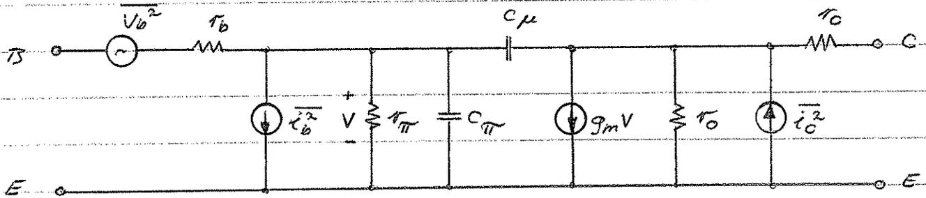
1.  $\overline{V_b^2} = 4kT r_b \Delta f$  due to base series resistor  $r_b$  (Thermal)
