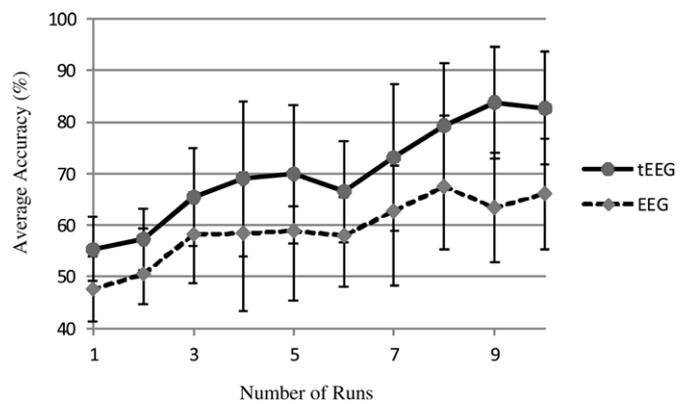
**Figure 5.** Average accuracy for tripolar concentric ring electrode (TCRE) (continuous line) and disc electrode (dashed line). The values are mean  $\pm$  SD.
