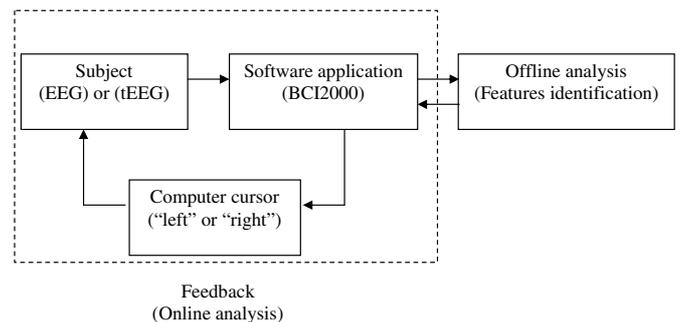
**Figure 3.** Procedure of one-dimensional computer cursor control.
