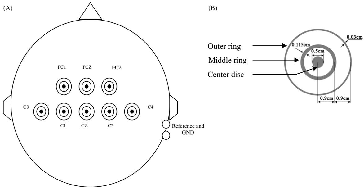
**Figure 1.** (A) Schematic illustration of the electrode montage. The EEG signal is recorded from the outer ring of the TCRE electrodes. EEG and tEEG signals were recorded from the same location concurrently. (B) Schematic of TCRE electrode.
