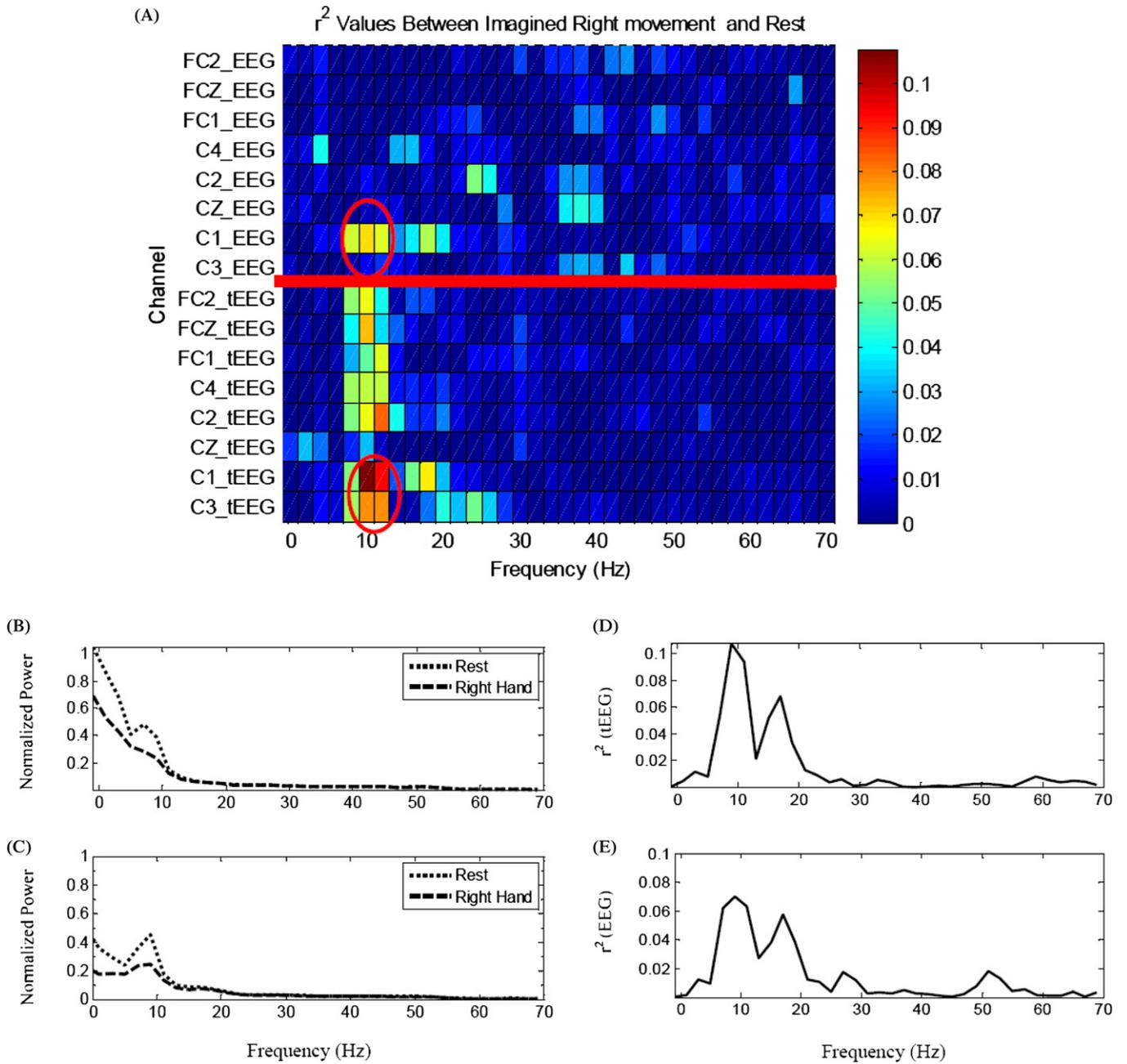
**Figure 4.** Example of an analysis comparing between tEEG and EEG signals for the ‘right’ hand imaginary and rest. (A) Values of  $r^2$  for all the electrodes locations and frequencies for both tEEG and EEG signals. Normalized power from channel C1 for (B) tEEG and (C) EEG. The corresponding  $r^2$  spectrum measures the amplitude variation for (D) tEEG (E) and EEG for electrode C1.
