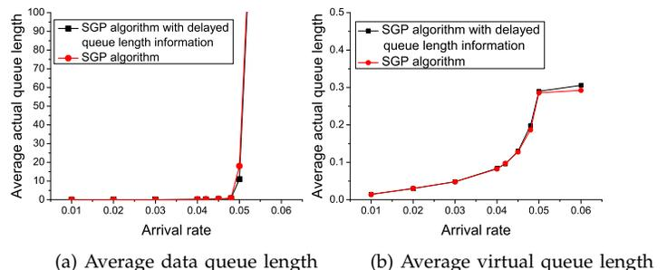
Fig. 6: Impact of using delayed queue length information
