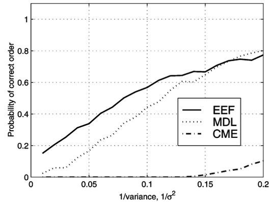
Fig. 5. Probability of correct model order for sinusoids versus inverse noise variance.
