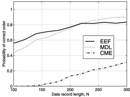
Fig. 4. Probability of correct model order for sinusoids versus data record length.
