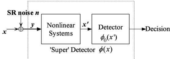
Fig. 10. An illustration of a SR detection system and the corresponding “Super” detector.
