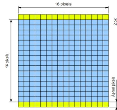
Figure 5: Position of apron pixels (yellow) and writable pixels (blue) in shared memory blocks for the vertical derivative
