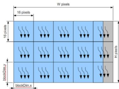
Figure 3: Division of work between threads in the naive GPU implementation. The gray area represents idle threads within the block.
