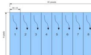
Figure 2: Division of work between threads in the CPU implementation.
