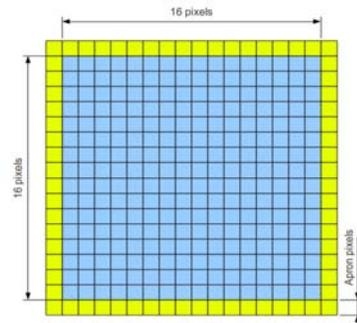
Figure 4: Position of apron pixels (yellow) and writable pixels (blue).
