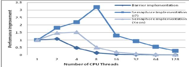
Figure 8: Performance of two different multi-threaded implementations of the Seam Map.
