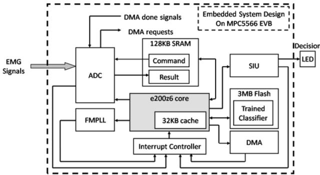
Fig. 3. Block diagram of embedded system design on MPC5566 EVB for real-time testing. MPC5566: device modules; ADC: analog-to-digital converter; FMPLL: frequency modulated phase-locked loop; SRAM: internal static RAM; SIU: system integration unit; DMA: direct memory access.
