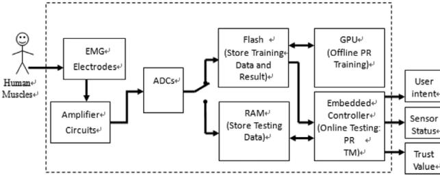
Fig. 2. Hardware architecture of designed neural-machine interface.
