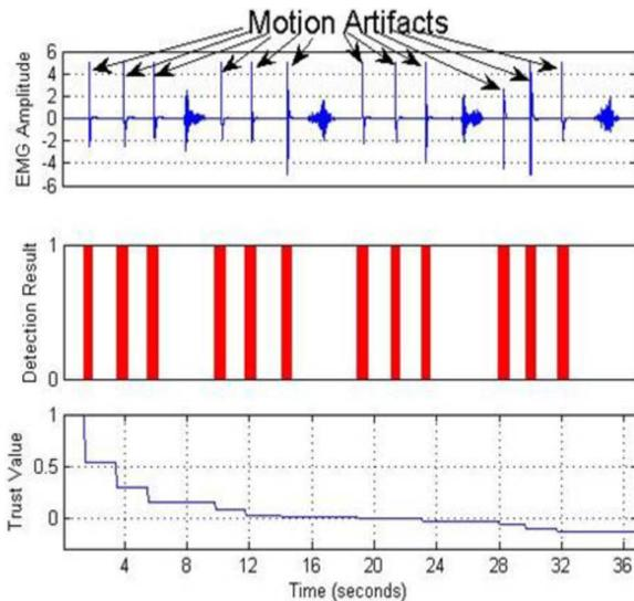
Fig. 7. Real-time performance demonstration of the abnormal detector under motion artifacts. The representative EMG signals (upper panel), the detection results of CUSUM (middle panel), and the trust value (lower panel) are demonstrated.
