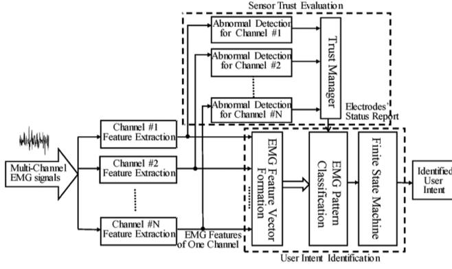
Fig. 1. Software architecture of EMG-based neural-machine interface for artificial legs.
