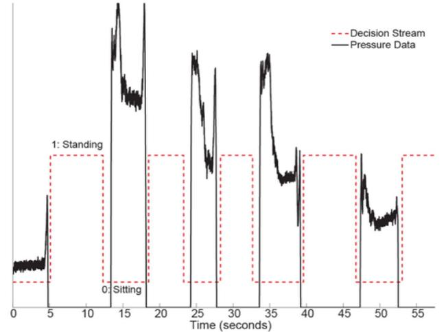
Fig. 5. Real-time performance of the designed NMI system. The decision stream (0: sitting, 1: standing) is aligned with the pressure data (black solid line) measured under the gluteal region of the subject.
