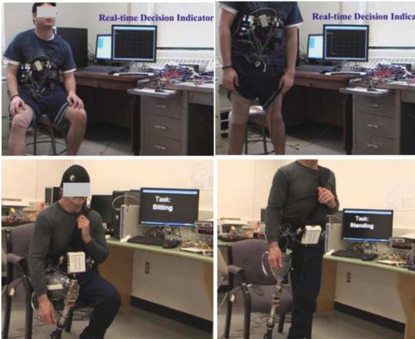
Fig. 6. Real-time testing of the designed NMI prototype on one patient with transfemoral amputation (lower two photos). Upper two photos show our experiments on an able-bodied subject.
